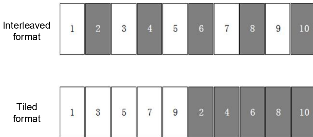
Figure D.9 Audio separation principle
