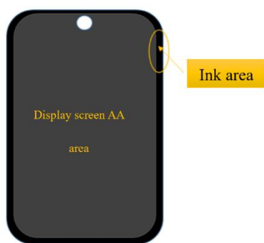
Figure 1 Schematic diagram of the display area (AA area) and ink area on the display screen
